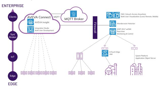
This example features a Unified Operations Management Center with a Command and Control room. Several distributed sites communicate with MQTT via cell modems. Additional sensors added at large sites communicate via high speed internet, distributing computing power to the edge and reducing latency. System Platform Monitors, Controls, Manages the Edge nodes.
