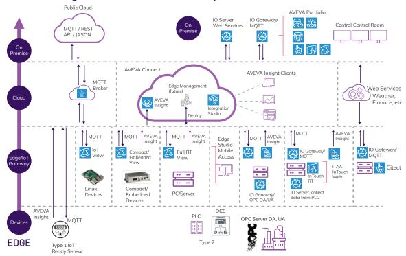
This scenario can include different types of edge devices. IoT ready devices can collect data from their sensor and publish directly to a cloud like AVEVA Insight, MQTT Broker, or a proprietary cloud. The other type might be an intelligent device typically connected to PLC/DCS or any OPC Server. Edge single node devices use native communication wherever possible, speaking to each device in its own language.
