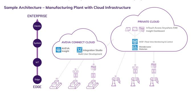
This architecture demonstrates a "Cloud First Strategy" which moves the infrastructure to the cloud, both with AVEVA Connect Cloud and virtual hardware residing in a private corporate cloud environment owned and maintained by the IT department. This scenario includes System Platform Running on Integration Studio Server (Development, Runtime Historian) and connected to real I/O via VPN secure connections. IoT sensors are added to existing lines/equipment and talk to the MQTT broker.
