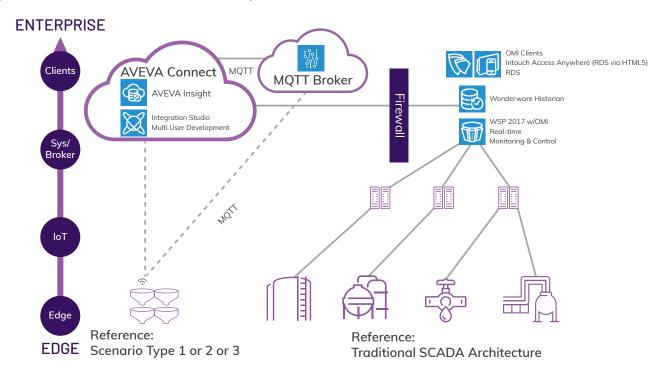
This traditional SCADA architecture utilizes on-premise System Platform & OMI servers. Existing PLCs and new edge sensors are introduced at key processes for monitoring only. Wonderware Historian provides data to AVEVA Insight, and AVEVA Connect / AVEVA Insight combines process plant and new sensor data.
