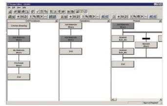
materials management as part of recipe procedure development. An InBatch master recipe may or may not be size specific, and can be assigned to any process line that has fits the equipment requirements defined in the recipe. All formula quantities for ingredients, intermediates, byproducts, and finished goods are configured as either actual quantities or scalable as a percent of the batch size.
