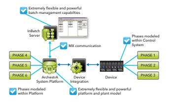
**Connectivity** – InBatch offers connectivity to any control system or plant floor device through Wonderware DA Servers. External databases and other software systems can be connected through ArchestrA System Platform.
